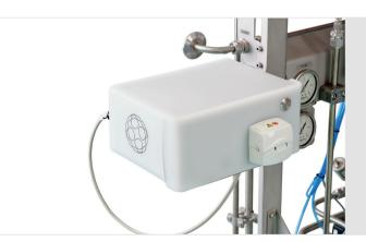
The Variable Speed Pump (bVSP) is the module you need when expanding the number of freely assignable pumps to cover multiple additions or withdrawal / harvesting actions according to a number of feeding / bleeding profiles or advanced controls.
